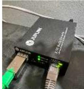
Gambar 3. converter fiber to RJ45
