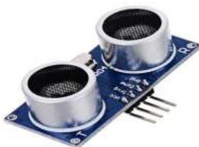
Gambar 2. Sensor Ultrasonik
