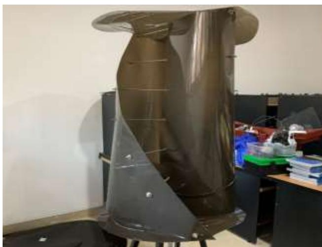
**Gambar 1.** Turbin savonius heliks.
